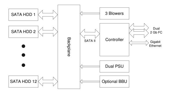
Figure 2-1: Raidtec FS3102 Block Diagram
